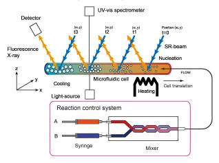
Figure 1: Schematic principle of in-situ XAS
